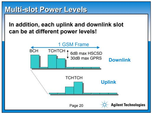
HSCSD and GPRS are both required to support timeslots at different power levels. Each timeslot on the uplink and downlink can be a different power level.
