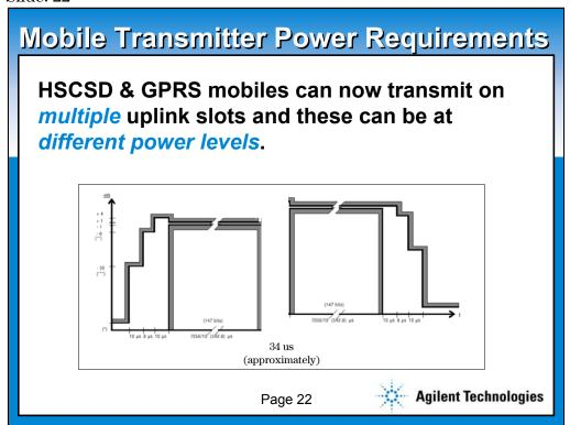
A new multislot Power versus Time mask has been defined for mobile and base station transmitters.
