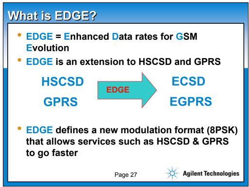
EDGE (Enhanced Data Rates for GSM Evolution) is an extension to HSCSD and GPRS that provides a further data rate increase.
