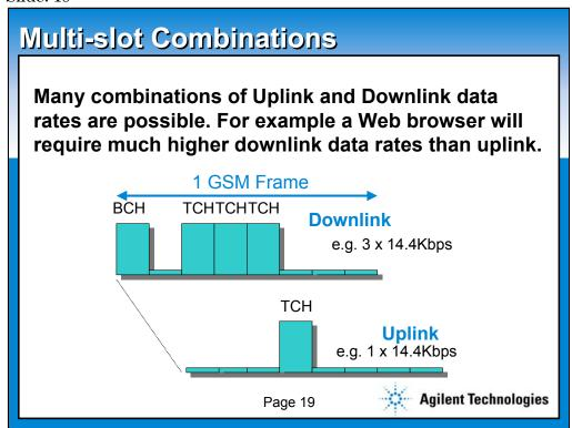
Depending on the type of data application that is being used the timeslot configurations of the uplink and downlink can be different. They can also be dynamically changed during the call depending on data application requirements and network capacity.
