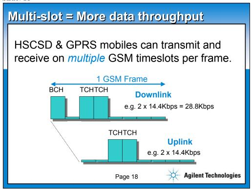
Using multiple timeslots per user allows the data rate to be multiplied up to 28.8kbps (2 slots), 43.2kbps (3 slots) or 115.2kbps (8 slots).
