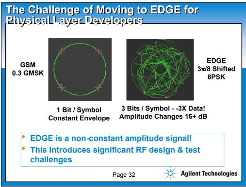
Because EDGE signals are non-constant amplitude GSM developers are faced with new design and test challenges. EDGE signals are inherently more sensitive to, for example, non-linear amplifier behavior and other component imperfections.
