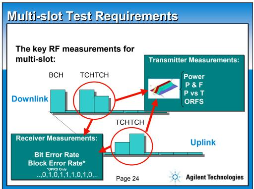
The important RF measurements for HSCSD & GPRS are almost identical to those used for standard GSM.
