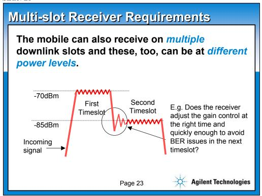
One of the key challenges of HSCSD & GPRS is designing a receiver that is capable or receiving adjacent timeslots that are at widely different power levels. This is more of an issue for GPRS since the max power difference between slots can be 30dB, compared to 6dB for HSCSD.
